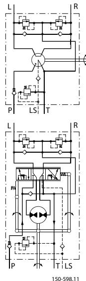
**OSPF LS : Steering unit full drain load sensing dynamic and with integrated valve functions**
