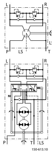
***OSPBX LS, OSPCX LS and OSPLX LS: Steering units load sensing for flow amplifiers***
