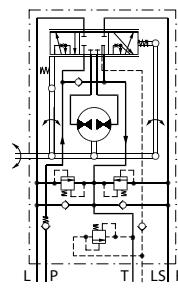
**OSPC LSR: Steering unit load sensing dynamic with integrated valve functions**
