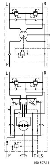
**OSPD LS: Steering unit load sensing dynamic with 2 rotary meters and with integrated valve functions**
